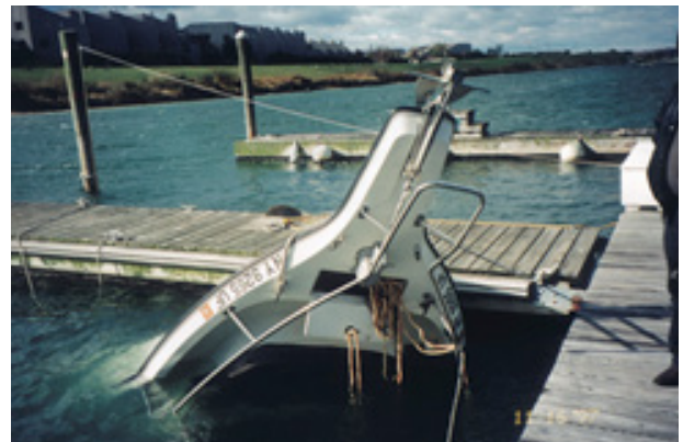
Most boats sink at the dock, like this center console that went under due to a failed hose clamp.
